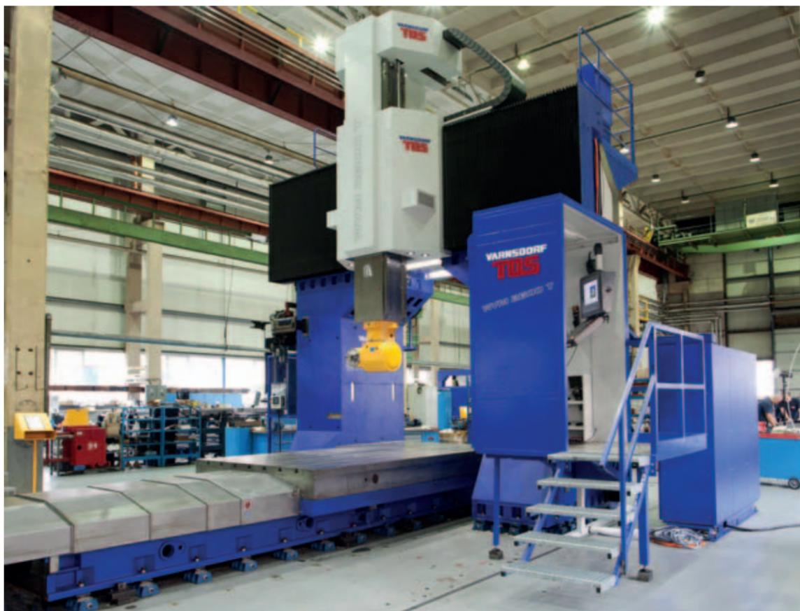
The WVM 2600 / 3600 T machine is a new table version of the portal machine. It is designed for accurate and highly productive coordinate milling, drilling, boring, and thread cutting especially into large and heavy workpieces or shaped workpieces from cast iron, cast steel, and steel.
